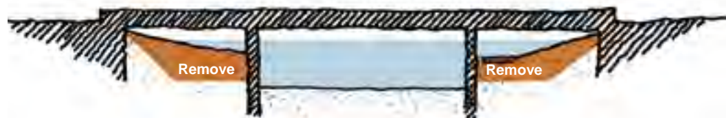
Proposed Modification – Increase Underpass Stormwater Capacity
